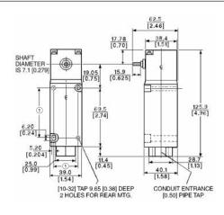
Can accommodate both U.S., 29.4 (1.16) x 59.5 (2.34) and DIN, 30 (1.18) x 60 (3.26), mounting dimensions.
